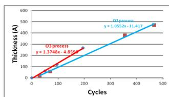
The chart shows the growth rate of ALD Pt/O<sub>3</sub> process and ALD Pt/O<sub>2</sub> with Al<sub>2</sub>O<sub>3</sub> as the nucleation layer at 250 °C. ALD Pt/O<sub>3</sub> process shows very little nucleation delay while ALD Pt/O<sub>2</sub> process shows 11 cycles of nucleation delay. The ALD Pt/O<sub>3</sub> process shows the growth rate of 1.37 Å/cy while the O<sub>2</sub> process shows the growth rate of 1.03 Å/cy.
