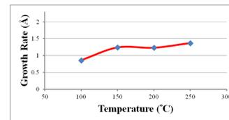
The picture depicts the variation of Platinum growth rate with process temperature for the O<sub>3</sub> process. As evident from the graph, the process shows ALD characteristics by exhibiting a constant growth rate across a wide range of temperatures.
