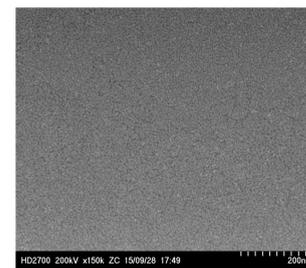
By STEM image of ALD Pt films on top of UV/ozone treated Si substrate, the Pt film is very smooth and the grain size is very small. It indicated that at a low temperature of 150 °C ALD Pt/O<sub>3</sub> has very good nucleation on SiO<sub>2</sub>/Si surface. In contrast, ALD Pt/O<sub>2</sub> process has a very long nucleation delay on SiO<sub>2</sub>/Si surface. The white bar on the bottom of each image represents 200 nm.
