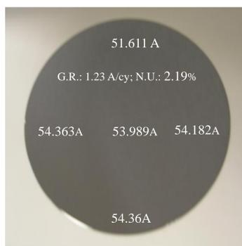
ALD Pt by O<sub>3</sub> process at 150°C on 200mm (8") bare Si wafer through exposure mode. The non-uniformity is around 2%.
