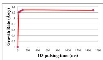
The left chart shows the saturated growth of Pt films versus pulsing of O<sub>3</sub> gas at 150 °C. Saturation curve shows that platinum growth saturates at 150ms O<sub>3</sub> pulse time. At dose lower than 40 ms, the growth rate is lower. The saturated growth is around 1.24 Å/cy. At this temperature there is very little Pt growth using pure oxygen.
