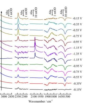
FIG. 2 IR spectra obtained during a cyclic voltammetric scan from -0.15 V to -1.4 V at the copper film electrode, Cu-Feb, deposited on a silicon prism in CO<sub>2</sub>-saturated 0.1 mol/L NaHCO<sub>3</sub>. The scan rate is 5 mV/s. The long black arrow indicates the direction of the potential. Scan scale bars above each wavenumber segment indicate the segments respective absorbance scale. The reference potential is -0.15 V.
