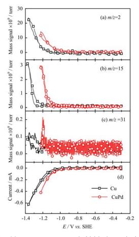
FIG. 6 Mass spectrometric signal of (a) hydrogen (m/z=2), (b) methane (m/z=15), (c) methanol (m/z=31), and (d) the measured Faradaic current corresponding to CO reduction on polycrystalline Cu (black line) and CuPd (red line) during a CV scan in CO-saturated 0.1 mol/L NaHCO<sub>3</sub> carried out at 10 mV/s.
