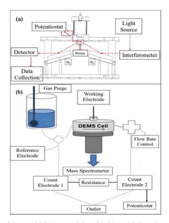
Scheme 1 (a) Schematic of the cell-holder and light path for *in-situ* electrochemical ATR-FTIR spectroscopy measurements. (b) Schematic for solution flow path used for DEMS experiments. Arrows represent the path of solution flow, and black lines represent wires connecting the various parts of the electrochemical cell.
