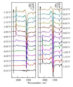
FIG. 4 IR spectra obtained during a cyclic voltammetric scan from -0.15 V to -1.4 V at a CuPd film electrode deposited on a silicon prism in CO-saturated 0.1 mol/L NaHCO<sub>3</sub>. The scan rate is 5 mV/s. The long black arrow points the direction of the potential. Scan scale bars above each wavenumber segment indicate the segments respective absorbance scale. The reference potential is -0.15 V.
