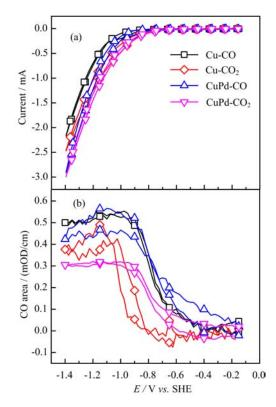
FIG. 5 (a) IR band integrals of the CO stretching vibration and (b) the faradaic current, measured during a CV scan Cu and CuPd film working electrodes in CO- and CO<sub>2</sub>saturated 0.1 mol/L NaHCO<sub>3</sub> carried out at 5 mV/s.
