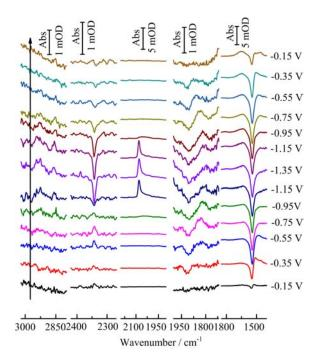
FIG. 1 IR spectra obtained during a cyclic voltammetric scan from -0.15 V to -1.4 V at the copper film electrode, Cu-Jun, deposited on a silicon prism in CO<sub>2</sub>-saturated 0.1 mol/L NaHCO<sub>3</sub>. The scan rate is 5 mV/s. The long black arrow indicates the direction of the potential scan. Scale bars above each wavenumber segment indicate the segments' respective absorbance scales. The reference potential is -0.15 V.
