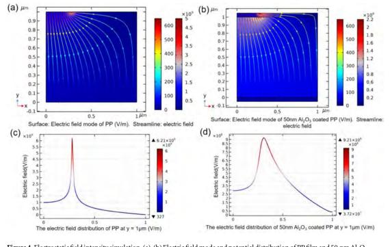
**Figure 4.** Electrostatic field intensity simulation. (a), (b) Electric field mode and potential distribution of PP film and 50 nm  $Al_2O_3$  coated PP film. (c), (d) One-dimensional electric field distribution of  $y = 1 \mu m$  of PP film and interface of 50 nm  $Al_2O_3$  coated PP film.
