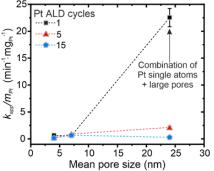
maximize catalytic activity of the composite material. It was found that instead of expected crystalline structure, Pt forms tiny 2D "rafts" that were previously found to be highly active in photocatalytic water splitting. In this work, the authors used the hydrogenation of 4-nitrophenol to quantify catalyst performance. A faster hydrogenation kinetics in samples with just one Pt ALD cycle, compared to multicycle Pt ALD, suggests that small Pt particles are more catalytically active.
